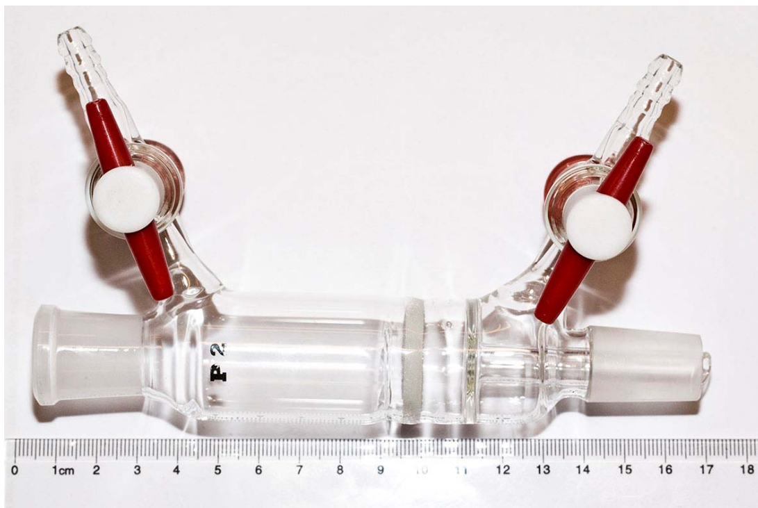
Equipment used for the inert (Ar) filtration of allylboronic acids 4a-i and 4l .
