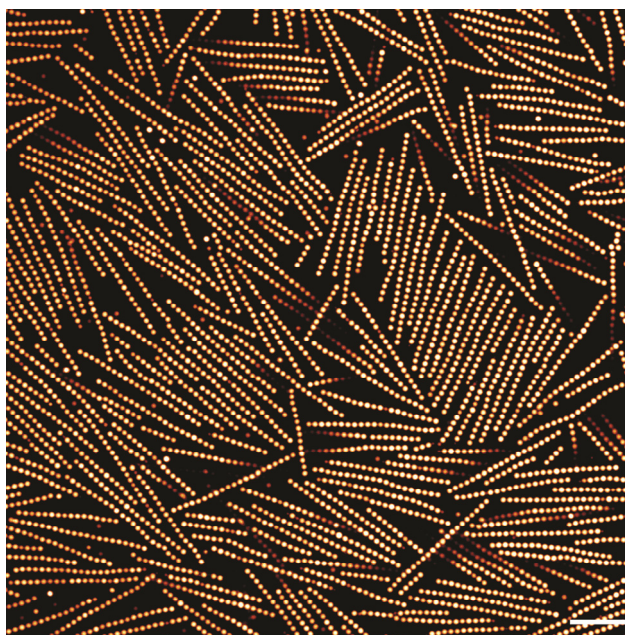
Fig. S1. Confocal microscopy image of 2D snapshot of permanent rigid PMMA chains in CHB. Scale bar, 5 \mu\text{m} .
