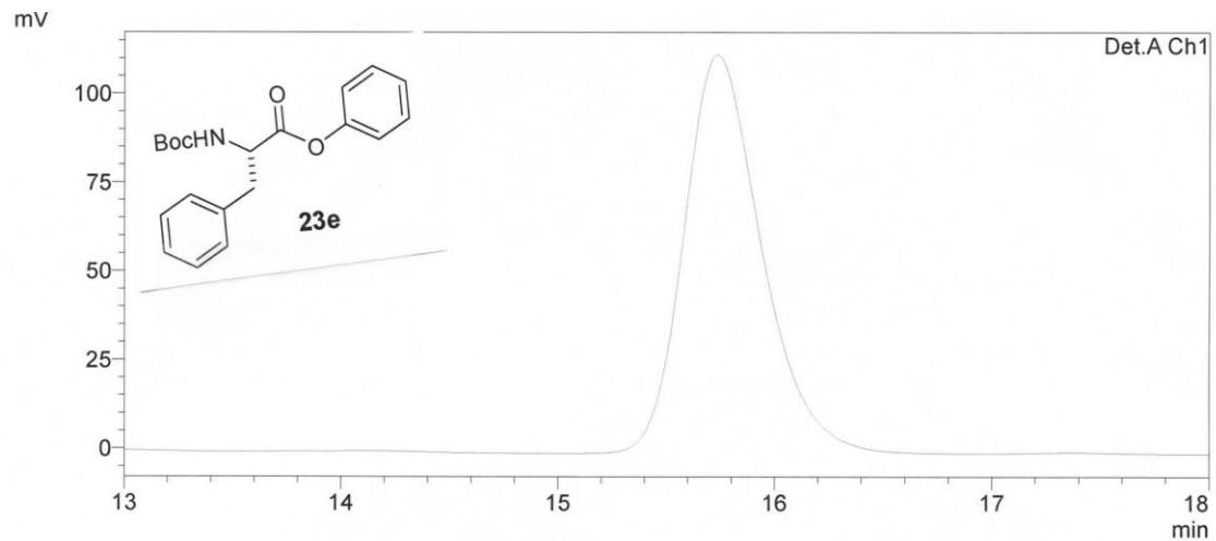
Chromatography condition:  $^i\text{PrOH:Hexanes}$  (30:70), Daicel Chiralcel OD-H column, 0.5ml/min, 254 nm
