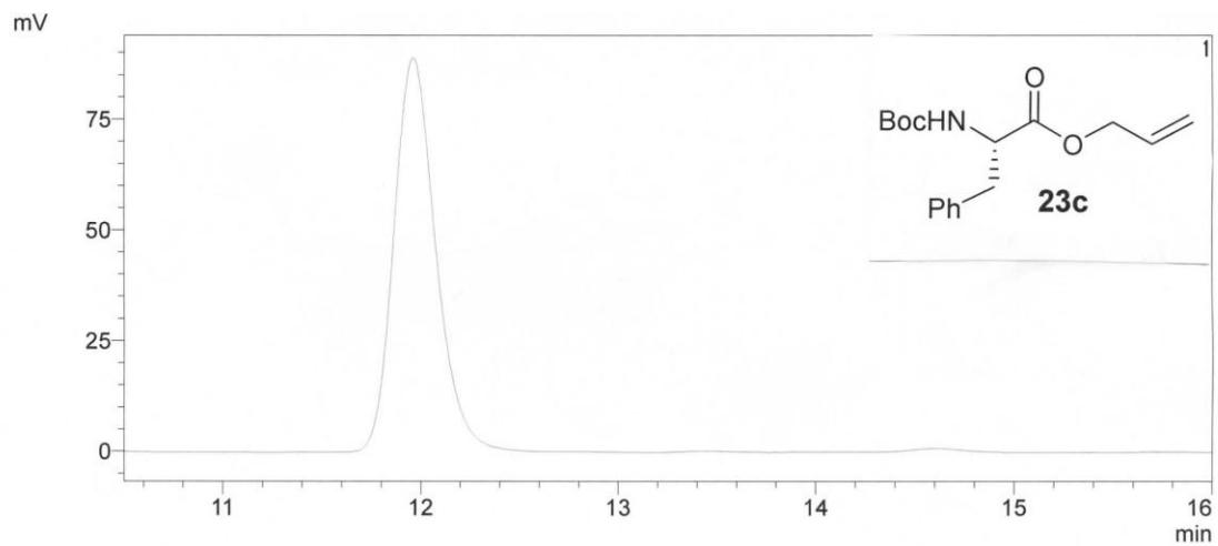
Chromatography condition:  $^i\text{PrOH}:\text{Hexanes}$  (30:70), Daicel Chiralcel OD-H column, 0.5ml/min, 254 nm
