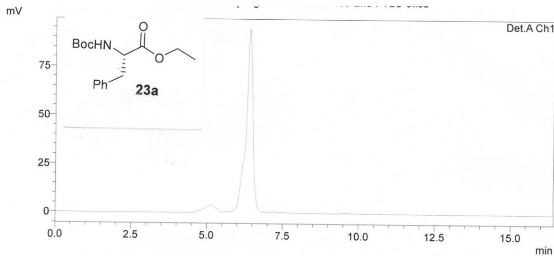
Chromatography condition:  $^i\text{PrOH:Hexanes}$  (30:70), Daicel Chiralcel OD-H column, 0.5ml/min, 254 nm
