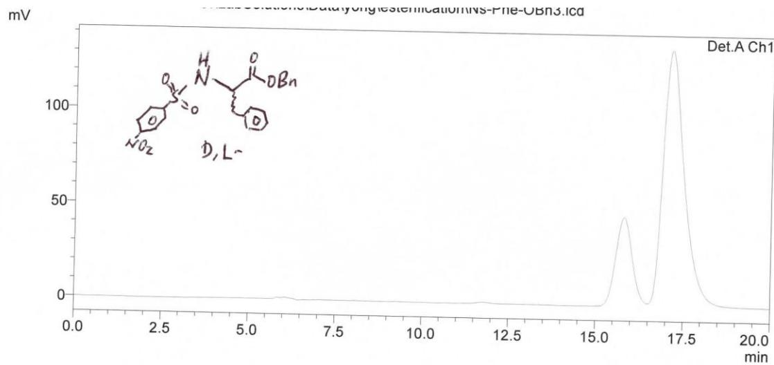
Chromatography condition:  $^i\text{PrOH}:\text{Hexanes}$  (30:70), Daicel Chiralcel OD-H column, 0.5ml/min, 254 nm
