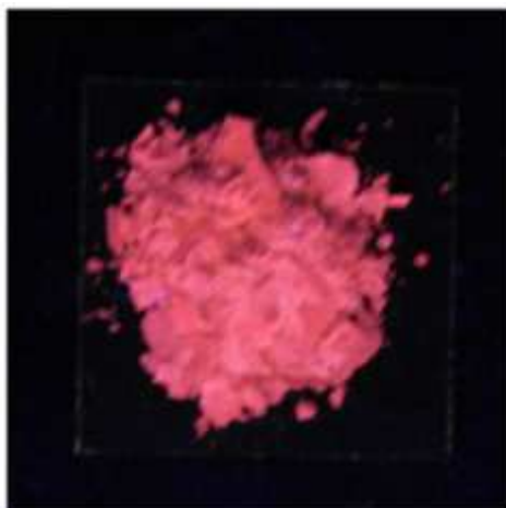
Figure S3. Photograph of the dried AuNPs/silica nanocomposites transferred from toluene/water interface, taken under UV light (365 nm).
