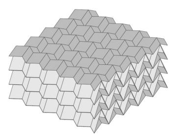
**Movie S1.** Individual Miura-ori sheets can be stacked together and bonded along joining fold lines to form a folded cellular metamaterial. Although the Miura-ori unit cell geometry varies between successive layers, the stacked configuration preserves the folding kinematics, and the 3D metamaterial expands/ contracts uniformly. Here, a stack with alternating layers *ABABABA* is shown.
