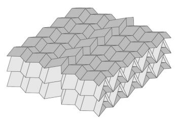
**Movie S2.** A self-locking folded cellular metamaterial. As the Miura sheets contract, the unit cells in the central column reach their maximum fold angle before the rest of the layer, thereby halting the folding motion and locking the metamaterial in a predetermined configuration. This behavior is achieved by varying the unit cell geometry within each layer.
