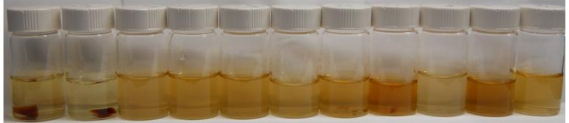
Figure S5. Digital images depicting the stability of hydrogels in water and aqueous EDTA.
