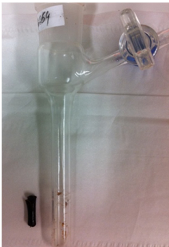
Figure S1. Photograph of the used Schlenk flask and the resulting monolithic Bet-PUR-2 material. The dark colour arises from impurities of the used Desmodur RE.
