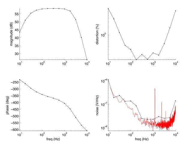
Check that the gain and cutoff frequencies are as you specified, and that the distortion and noise floor are < 1% and < 100 nV/rHz respectively.
