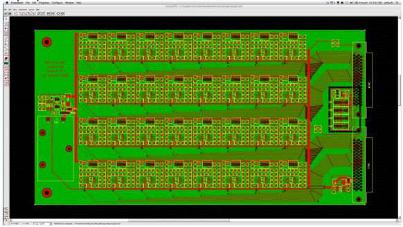
*amp32h.pcb* contains additional (and optional) hygrometer daughter boards. The main board includes space for one hygrometer, plus jacks for four remote boards. *amp2.pcb* (sic, not *amp32.pcb*) contains four hygrometers daughter boards in the layout, which can be removed from the board with a band saw.
