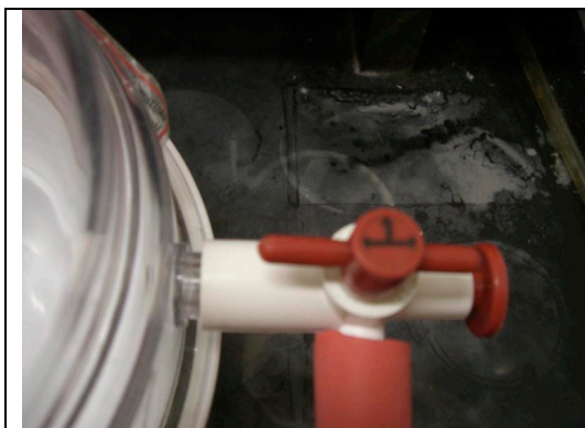
Fig. 1 Closed desiccator valve
