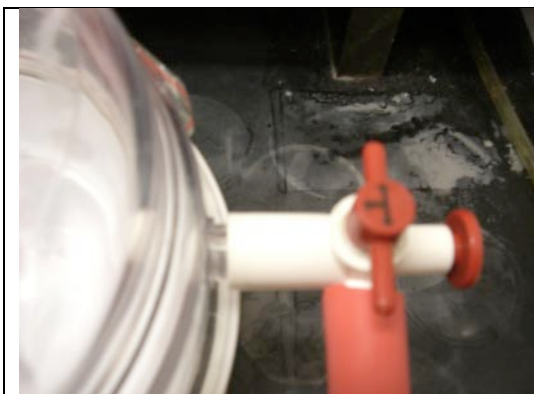
Fig. 2 Open desiccator valve
