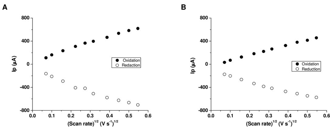
Figure 1. Dependence of the peak current ( $I_p$ ) as a function of the square root of the scan rate obtained with the OTCE fabricated with 12 layers of protein adsorbed/pyrolyzed for  $K_3Fe(CN)_6$  (A) and  $Ru(NH_3)_6Cl_3$  (B). Conditions: 1 mM for each electrochemical couple in 0.1 M  $NaH_2PO_4/Na_2HPO_4$  buffer + 0.1M KCl, pH = 7.4.
