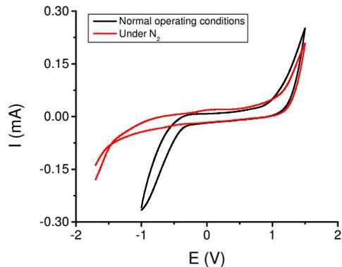
Figure 4: Electrodynamic profiles obtained with an electrode fabricated with 12 layers of protein adsorbed/pyrolyzed. Conditions: 0.1 M  $NaH_2PO_4/Na_2HPO_4$  buffer + 0.1 M KCl, pH = 7.4, scan rate:  $100\text{ mV}\cdot\text{s}^{-1}$ .
