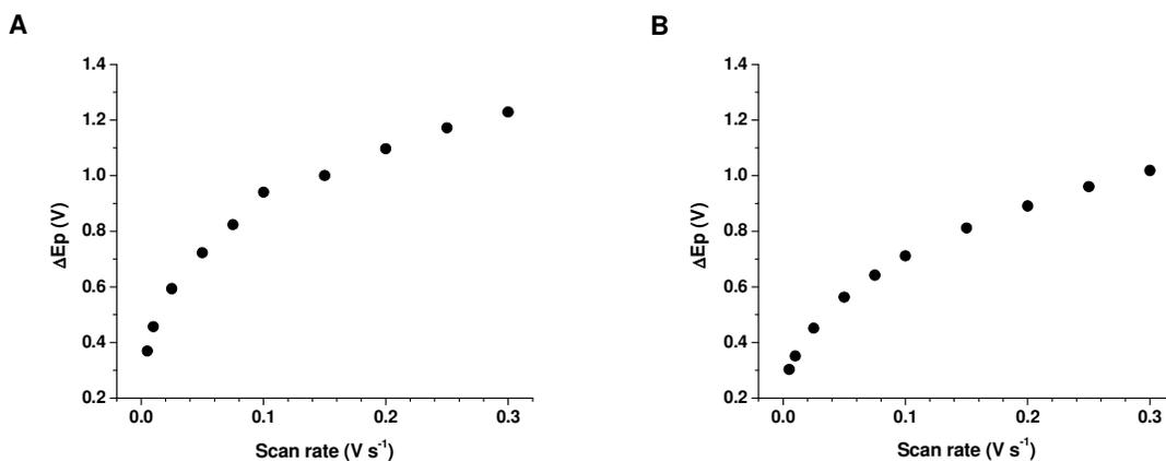
Figure 2. Dependence of the peak potential difference ( $\Delta E_p$ ) as a function of the scan rate obtained with the OTCE fabricated with 12 layers of protein adsorbed/pyrolyzed for  $K_3Fe(CN)_6$  (A) and  $Ru(NH_3)_6Cl_3$  (B). Conditions: 1 mM for each electrochemical couple in 0.1 M  $NaH_2PO_4/Na_2HPO_4$  buffer + 0.1M KCl, pH = 7.4.
