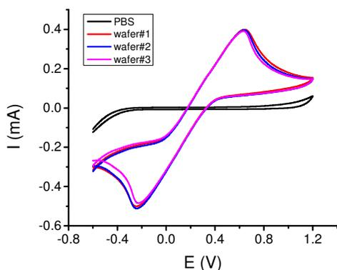
Figure 3. Electrodynamic profiles obtained with 3 electrodes fabricated with 12 layers of protein adsorbed/pyrolyzed. Conditions: 1.0 mM  $K_3Fe(CN)_6$  in 0.1 M  $NaH_2PO_4/Na_2HPO_4$  buffer + 0.1 M KCl, pH = 7.4, scan rate:  $100\text{ mV}\cdot\text{s}^{-1}$ .
