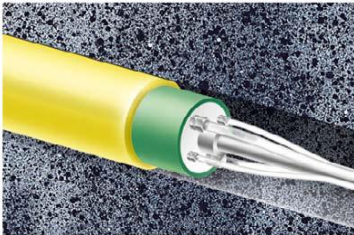
Supplementary Figure 1. The packer system: The yellow sections are expandable polyurethane packers, while the green rings are Teflon-coated stainless steel casings. The grey components are made of PEEK, as are the 1/8" (outer diameter) sampling tubes. Groundwater sampling and circulation are mediated via two small holes opposite each other in the grey portion in the middle of the packer assembly (the dark spot in the top drawing). The depicted section is 100 mm long.
