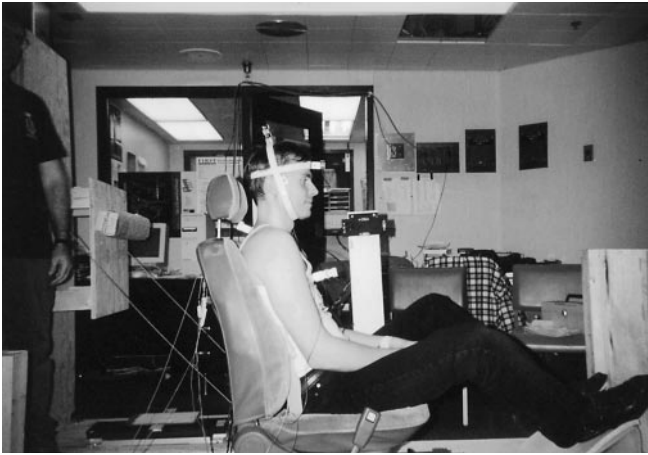
Fig. 1 The experimental set-up with a subject in a car seat on the sled. A head restraint was present but subjects never contracted it. Selspot markers and accelerometers parallel to the direction of motion were located on the sled, chest, and head
