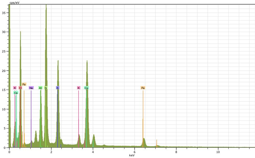
**Figure ESI-4C:** EDX spectrum obtained from Sample AT54A1-08
