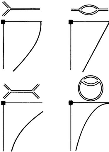
FIG. 5. Structure of replicating molecules affects the shape of the nascent strand arc. The situations shown, clockwise from top left, are *Bam*HI-*Bgl*II-restricted molecules with an origin to the right or left of the molecule, *Bam*HI-restricted molecules which contain an origin at the center, intact circular molecules, and *Bgl*II-restricted molecules which have a replication terminus at the center. The closed box and horizontal and vertical lines are explained in the legend to Fig. 1E.
