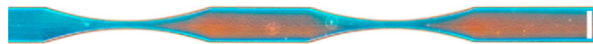
Fig. 55. Polarization microscopy reveals the flow behavior of polyethylenebutylene- b -ethylene oxide (PEB-PEO) micelles (30% wt/wt in water) in consecutive taperings. In this example, the micelles are pumped through a 250- \mu m channel with two 250- \mu m taperings at a rate of 300 \mu L/h. The flow orientation is from left to right. (Scale bar: 200 \mu m.)
