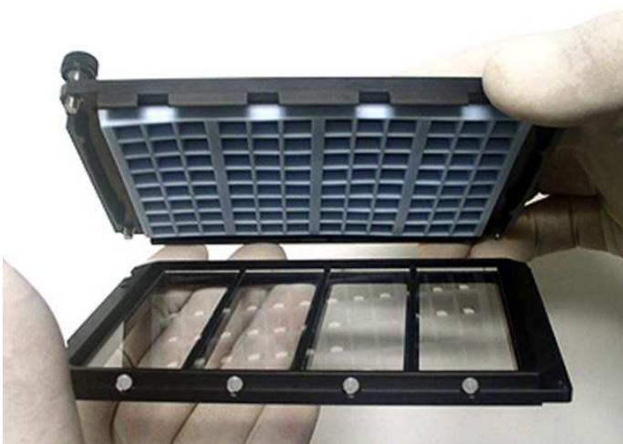
Picture 1. Slide assembly using MMH4x24 ArayIT kit.
