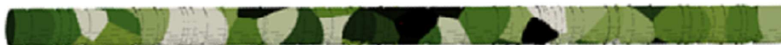
Figure S2. Simulation of the grains in a 85 nm diameter and 3.6 \mu\text{m} long Ni nanowire used to calculate the remanent magnetic state. Each part with different colors corresponds to different orientation of the crystalline anisotropy.
