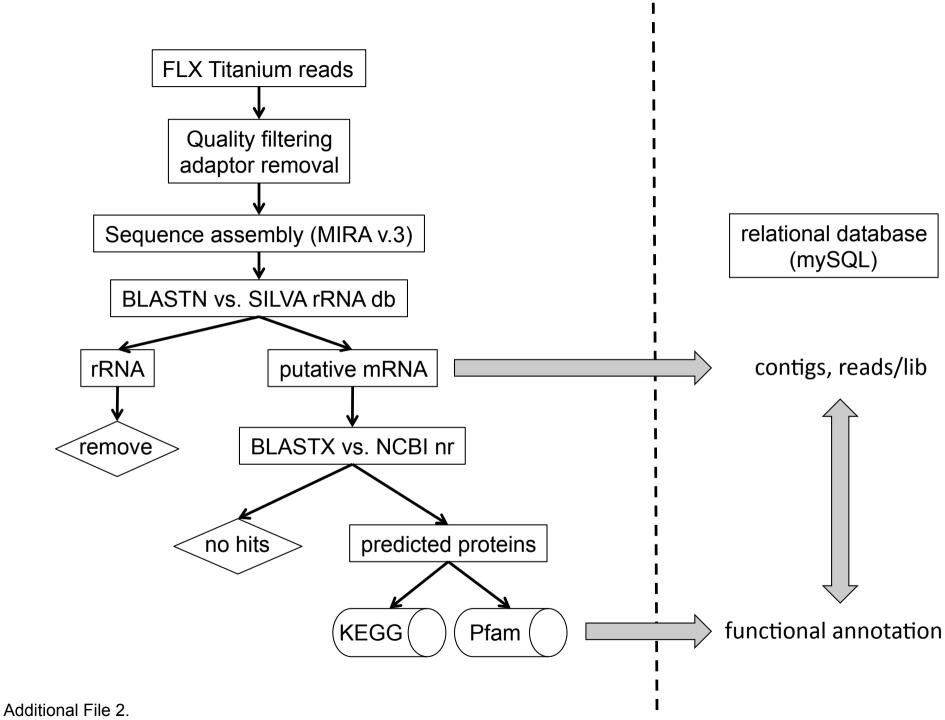
Flow-diagram showing the workflow for sequence quality assessment, assembly, annotation, and simple database structure.
