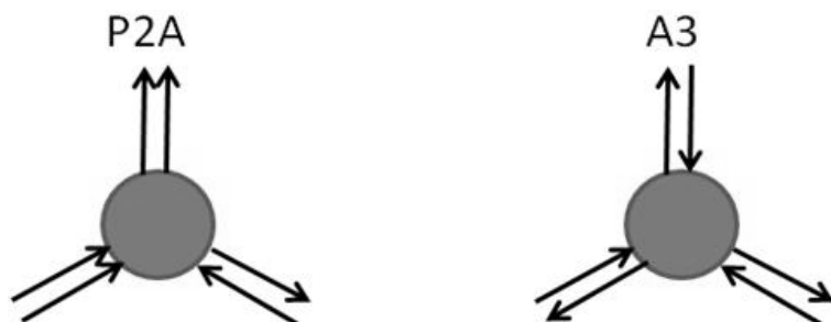
Supplementary Figure 3 | Two types of vertices existing in a cubic polyhedron. The number of incoming and outgoing helices have to be equal.
