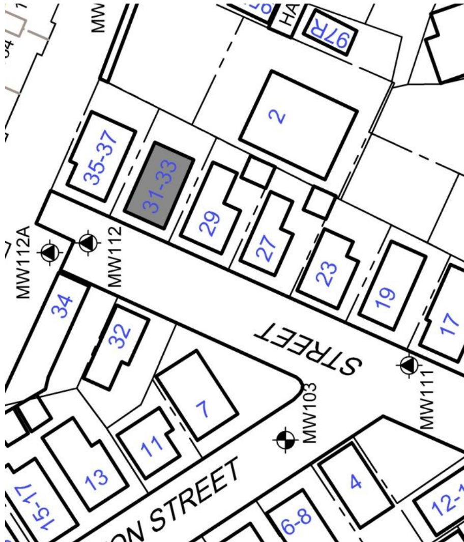
Figure 1. A portion of the site location showing the structure of interest. This is a residential neighborhood, consisting of many small parcels. The location of numerous groundwater monitoring wells is shown. Soil vapor was measured through the basement slab and indoor air concentration measured in the basement of the indicated building, which was located several hundred feet from the source area.
