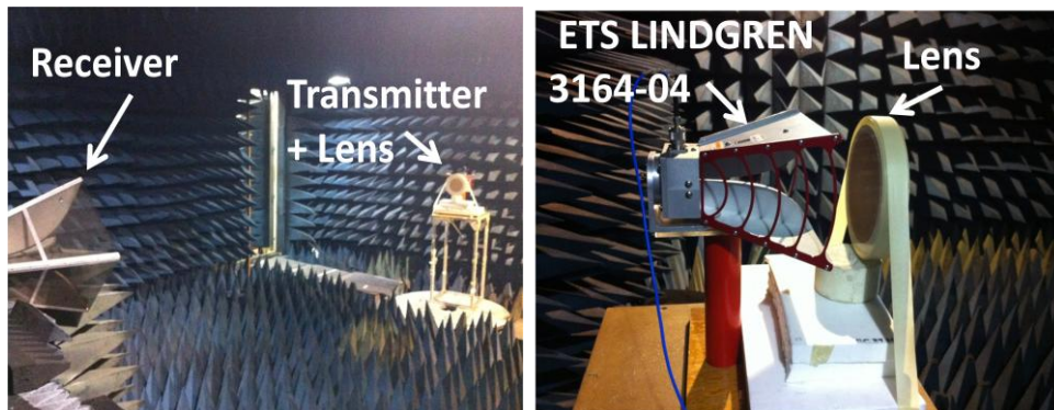
Figure S5 | Measured direct ray radiation pattern in an anechoic chamber. (a) 1-4GHz. (b) 5-7GHz. (c) Configuration in the anechoic chamber.
