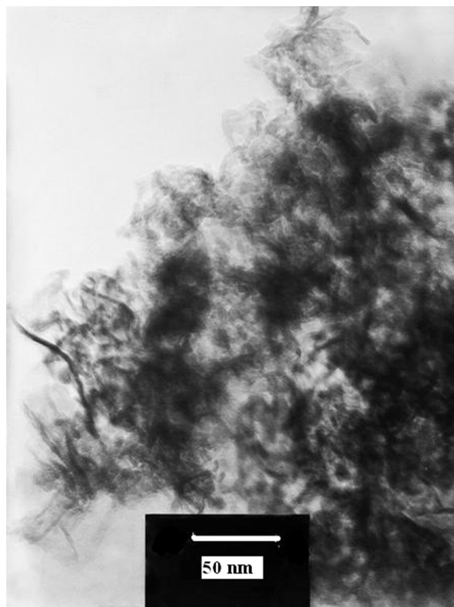
Fig. S3. Transmission electron microscopy (TEM) image of CaMnO shows layered structure morphology.
