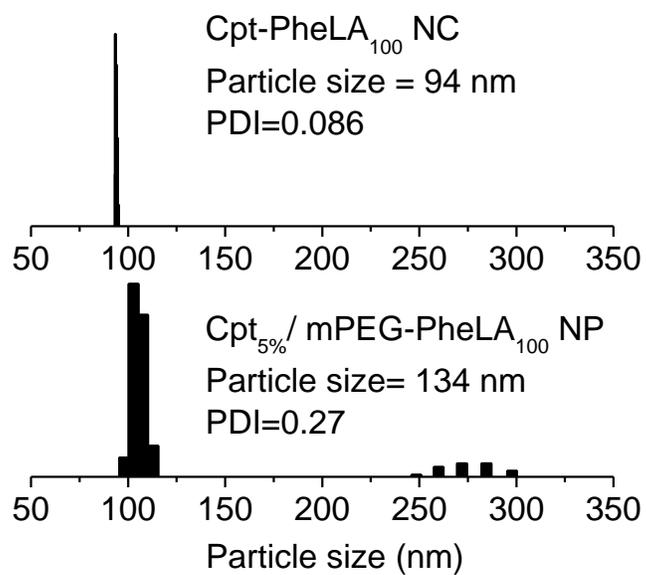
**Figure S5.** Dynamic light scattering (DLS) spectra of Cpt-PheLA<sub>100</sub> NCs prepared by nanoprecipitation in water (0.5 mg/mL) and Cpt<sub>5%</sub>/mPEG-PheLA<sub>100</sub> NPs prepared by encapsulation in water (0.5 mg/mL).
