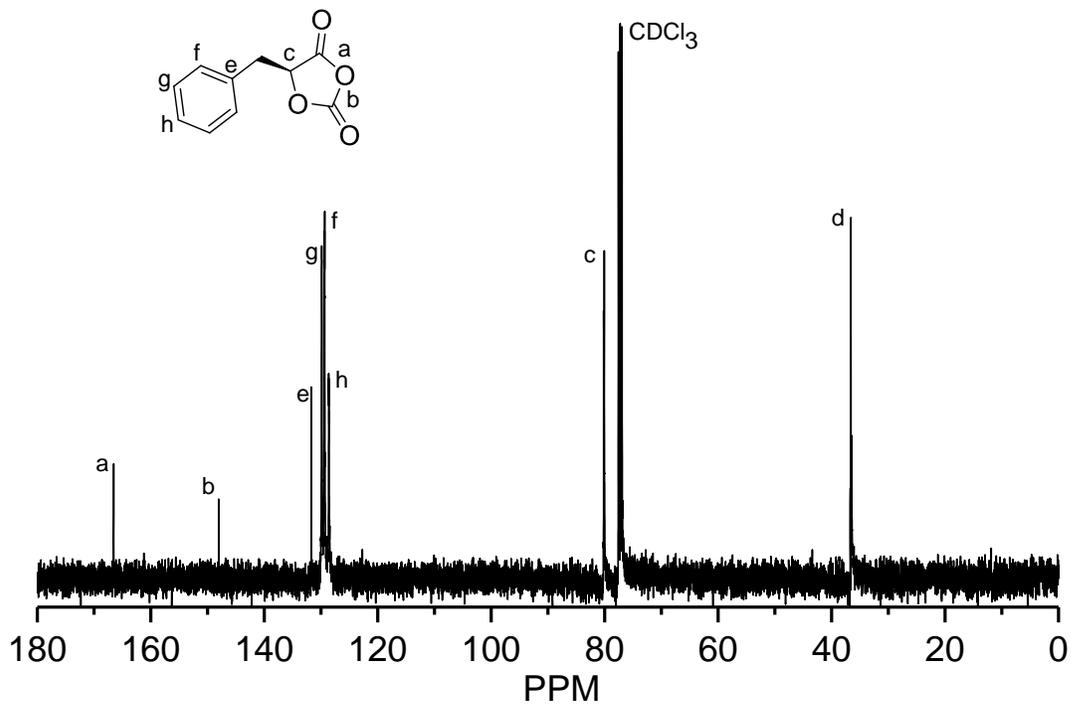
**Figure S2.**  $^{13}\text{C}$  NMR spectrum of Phe-OCA in  $\text{CDCl}_3$ .
