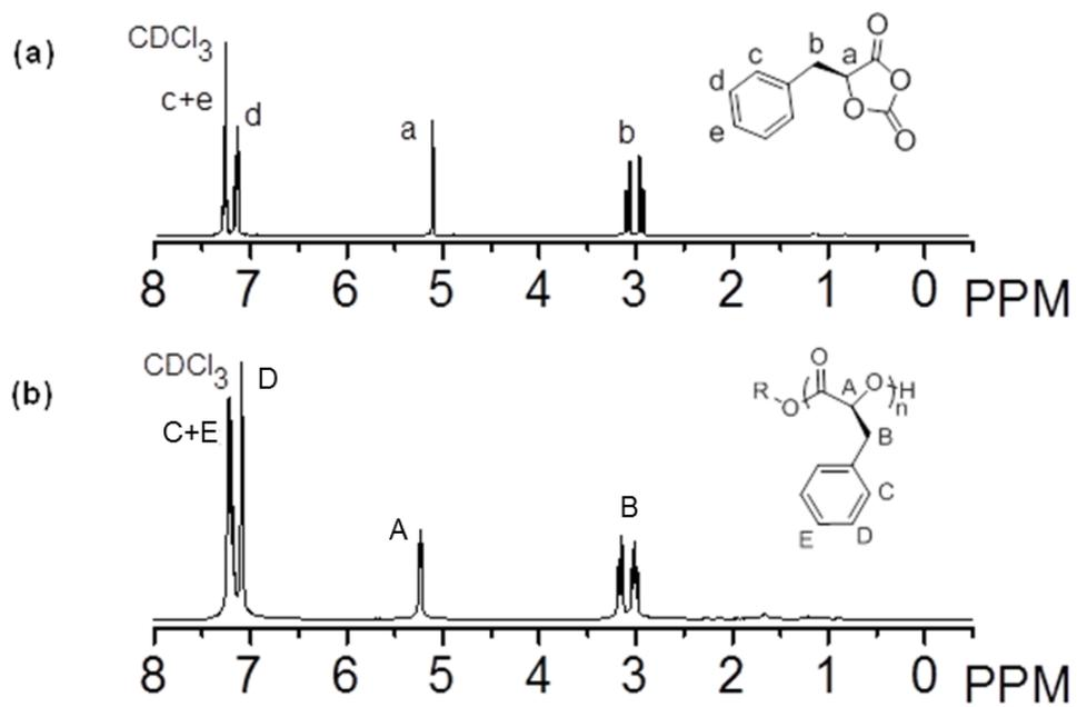
**Figure S1.**  $^1\text{H}$  NMR spectra of Phe-OCA (a) and poly(Phe-OCA)<sub>100</sub> (PheLA<sub>100</sub>) in  $\text{CDCl}_3$ .
