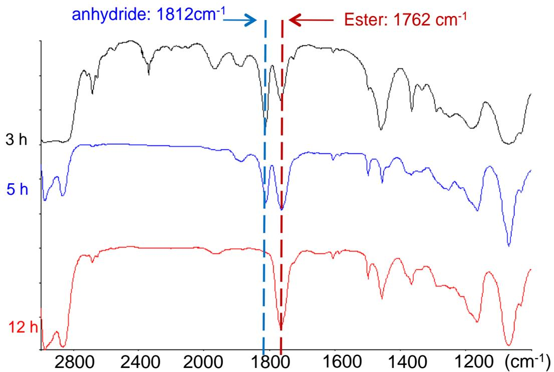
**Figure S3.** FT-IR spectra of Cpt initiated polymerization of Phe-OCA at 3 h, 5 h and 12 h.
