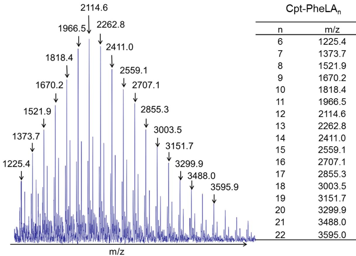
**Figure S4.** MALDI-TOF MS analysis of Cpt-PheLA<sub>15</sub>. The obtained  $m/z$  is identical to the calculated  $m/z$  of Cpt-PheLA<sub>n</sub> ( $348.35 + 148.2 \times n$ ).
