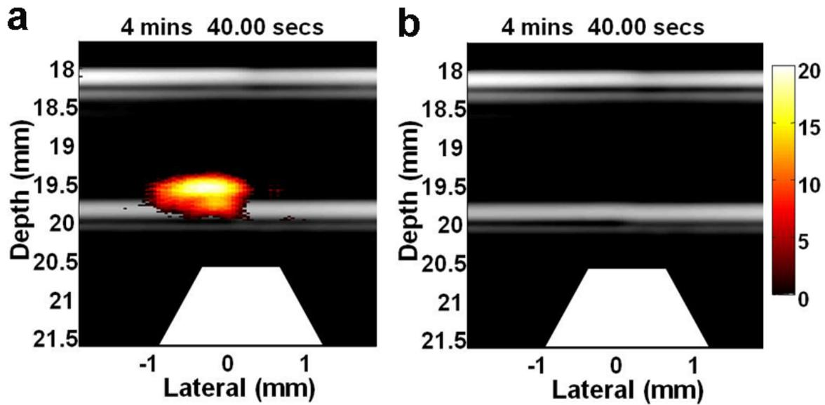
**Figure S3.** Combined US and PA images of captured HeLa cells labeled with (a) GNR-silica-MNP-FA (b) GNR-silica-MNP-FA together with 1 mM free folic acid in cell-culture plate. All the samples were measured at cell concentration of 5000 cells/mL.
