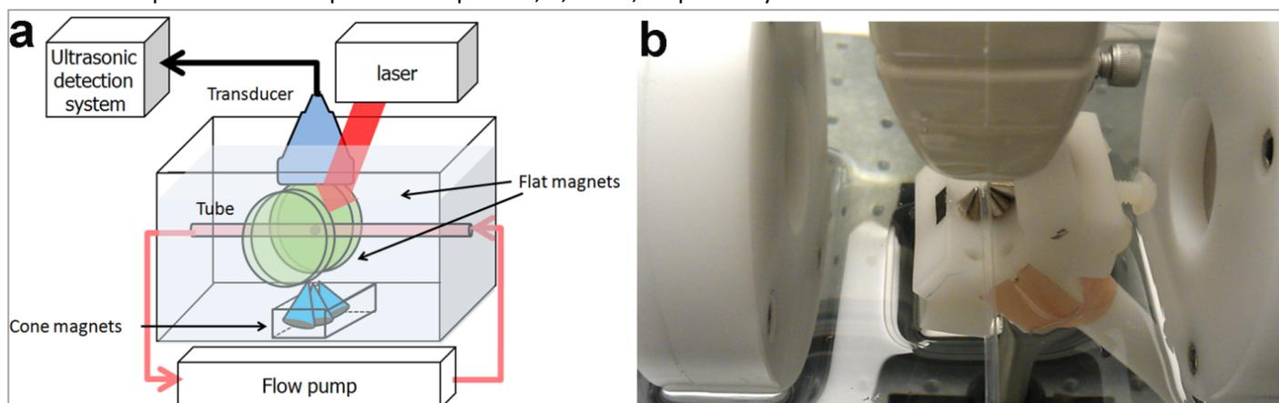
**Figure S2.** Schematic (a) and actual photo (b) of the CTC trapping and imaging system composed of a dual-magnet part, a continuous flow circulation part, an optical illumination head, and an US detector.
