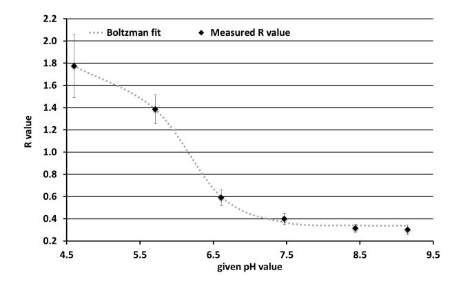
FIG. S4. A typical calibration response of the  $CO_2$  sensor and the corresponding Boltzman fit for  $CO_2$  calculation.
