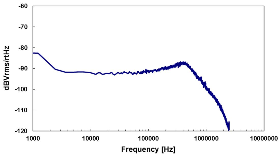
**Supplementary Figure S1.** Frequency spectrum of thermal fluctuations of a small cantilever (BL-AC10FS, Olympus, Tokyo, Japan) in water.
