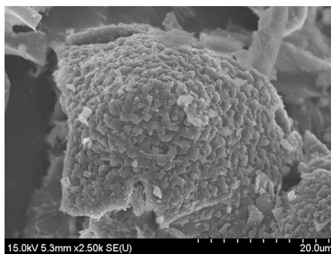
Fig. S3. SEM image of the RH-originated silicon obtained from the same synthetic procedure but with no acid treatment, indicating that the original nanoporous structure collapses if the acid treatment is omitted.
