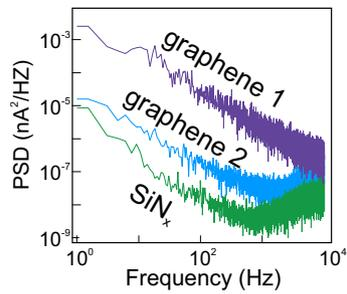
**Fig. S3.** Noise power spectral densities for three typical nanopores. Graphene 1, a 5-nm diameter nanopore in single-layer graphene suspended across a  $200 \times 200$ -nm  $\text{SiN}_x$  aperture; graphene 2, a 5-nm diameter graphene nanopore across a 20-nm diameter  $\text{SiN}_x$  aperture showing greatly reduced noise;  $\text{SiN}_x$ , a 5-nm diameter nanopore in  $\text{SiN}_x$  with no graphene.
