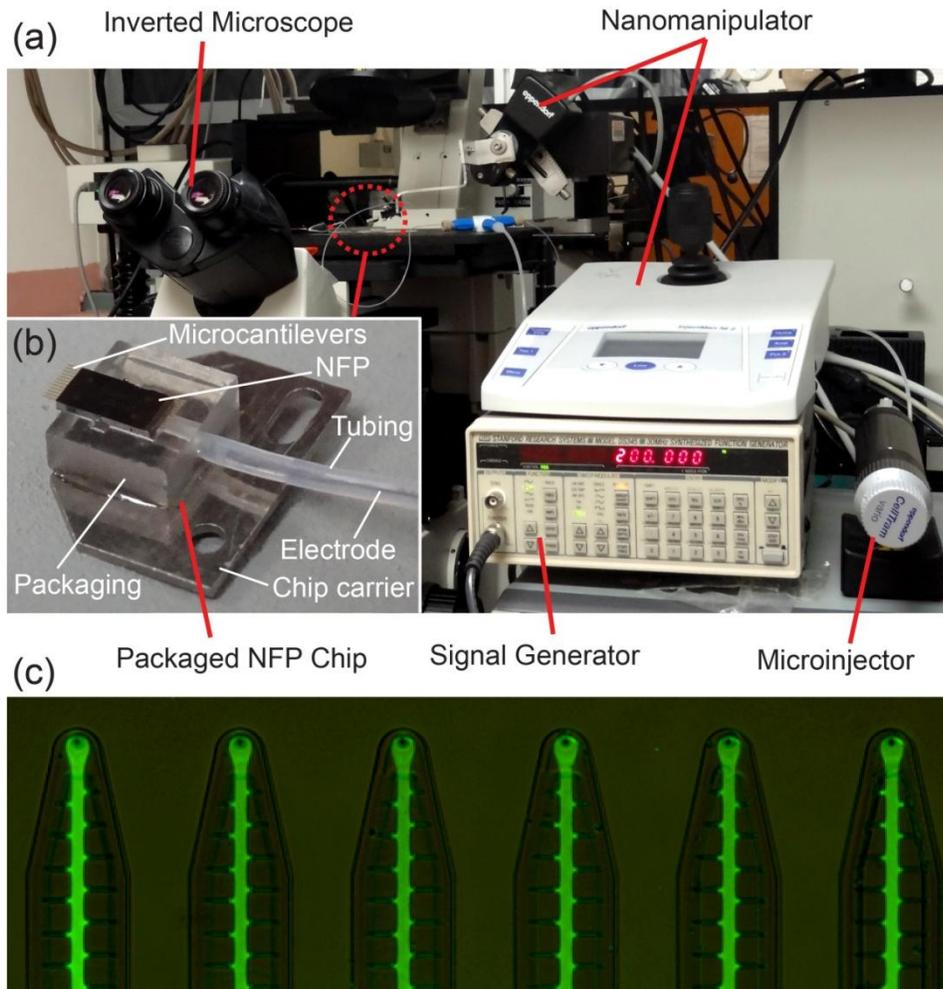
**Figure S1** NFP-E system: (a,b) Experimental setup including the packaged NFP chip mounted on the nanomanipulator on top of an inverted optical microscope, (c) Bright field optical microscope image merged with a fluorescence image of the NFP probes during wetting of the NFP microchannels with a solution containing Alexa Flour 488.
