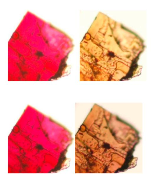
**Fig. S1** Pleochroitic behaviour of a single-crystal of **3+–CS2–** in linearly polarised light. The crystal is turned by 0° (top left), 90° (top right), 180° (bottom left) and 270° (bottom right).
