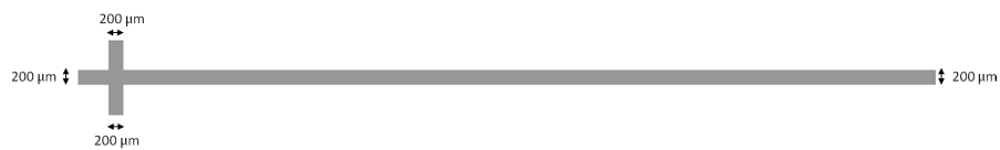
Figure 3. This is the scaled T-Channel geometry that was simulated and discussed in Section 4.1. The results of this simulation are shown in figure 4. The geometry consists of three perpendicular 200 \mu\text{m} wide inlets. Channel depth is kept constant at 50 \mu\text{m} , as is channel width ( 200 \mu\text{m} ), throughout the geometry. This T-Channel mixer has approximately the same pathlength as the SeLMA micromixer.
