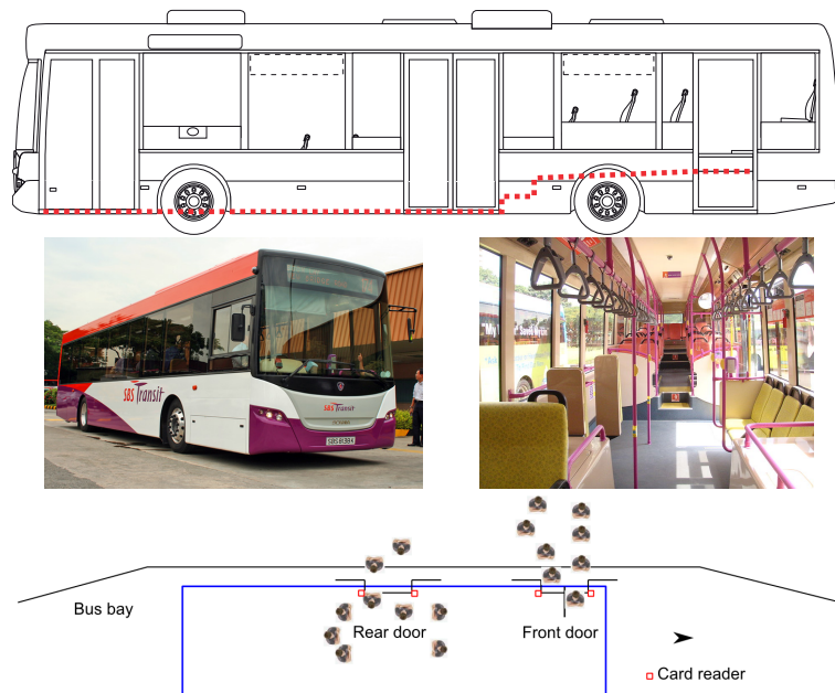
Figure S1: Layout of the Scania K230 single decker lower floor bus and location of smart the card readers
