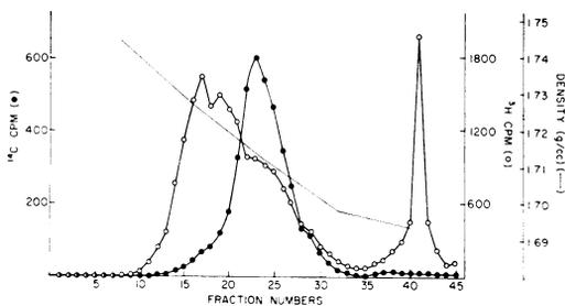
FIG. 3. Isopycnic CsCl centrifugation for 72 hr at 33,000 rev/min at  $20^\circ\text{C}$  in Spinco model 40 rotor. Newly released  $^3\text{H}$ -AAV-2 DNA and double-stranded  $^{14}\text{C}$ -AAV-2 marker DNA. The conditions of DNA release were those described in the legend to Fig. 2.
