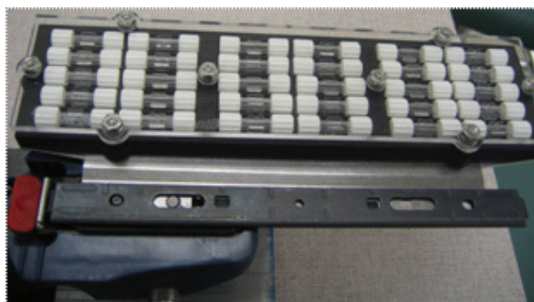
Figure S1. FineMix30 oscillator (Claremont BioSolutions), which allows simultaneous testing of up to 30 tubes for DNA bulk depletion experiments. The device oscillates linearly with tunable frequencies (up to 20 Hz). A photo tachometer was used to monitor the frequency of oscillation.
