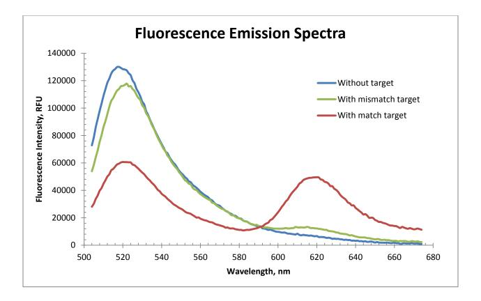
**Figure S2. Fluorescence resonance energy transfer demonstrated by fluorescence emission spectra**. 200 nM anchor (Oligo 1) and T-allele probe (Oligo 2) were incubated and measured at 37°C without target RNA (Blue line), with mismatch target Oligo 10 (Green line), and with match target Oligo 9 (Red line).
