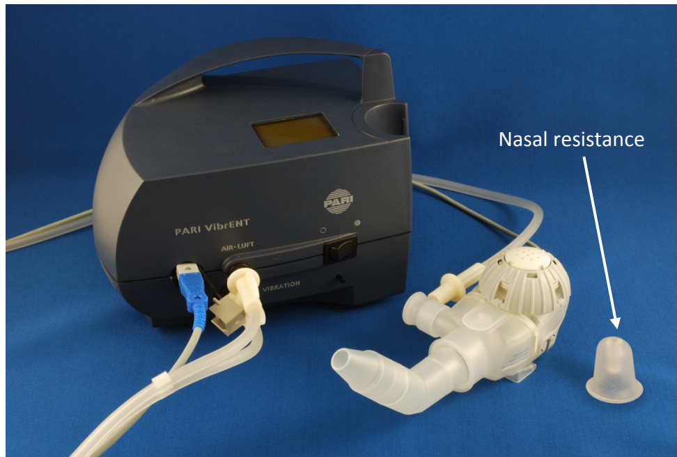
Figure S1: Prototype of the Vibrent® pulsating aerosol device consisting of a pulsating membrane nebulizer with nostril adaptor, flow and 25 Hz pulsation generator and the nasal resistance.
