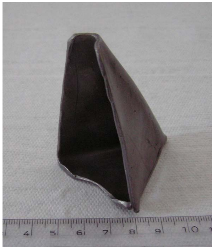
Figure S2: Lead mask for shielding the activity in the central nasal cavity during anterior imaging in front of the gamma camera. The lead mask consists of 2 mm lead causing an attenuation of the gamma rays by about a factor of \approx 900 .
