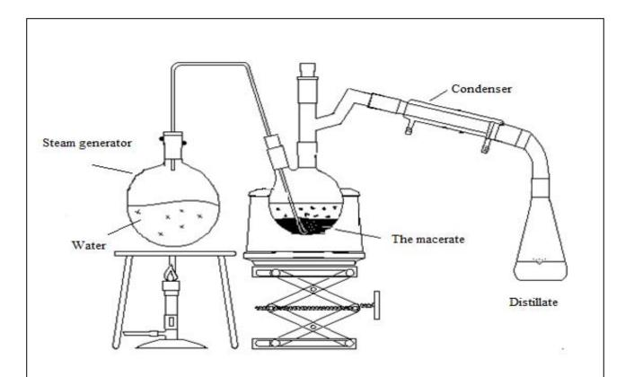
**Figure1: Steam distillation apparatus**; Vapors are formed by heating the water in the first round-bottomed flask, Steam produced are drawn into the glass tube, then leads the hydrocyanic acid released by maceration, in the second round-bottomed flask, vapors of HCN are condensed and trapped in silver nitrate.
