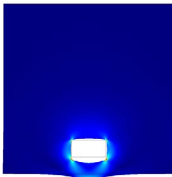
Fig S6. PDMS channel deformation at an applied internal pressure of 1 bar. The largest channel deformation is directed towards the thin bottom layer. PDMS channels extending into the bulk of the device contribute much less, c \approx 1 \cdot 10^{-15} \frac{m^2}{Pa} , but this is harder to estimate accurately due to complex device geometry.
