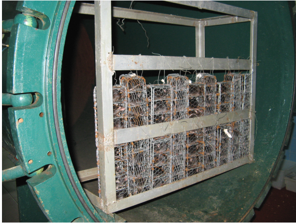
Supplementary Fig 2 Photo illustrating the BST-I apparatus and the position of the cage-array in the same vertical plane to ensure equal exposure to WBBI for all mice.
