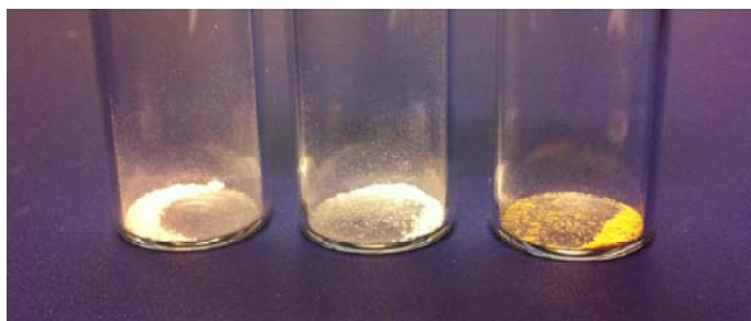
Figure S4. Photograph of pristine UiO-66 (left), UiO-66 after incubation with complex 2 and standard rinsing (middle), and UiO-66 after incubation with complex 1 and standard rinsing (right). Incorporation of 1 via PSE is evidence by the persistent color of the sample, indicating formation of UiO-66-[FeFe]dcbdt(CO) 6 (right).
