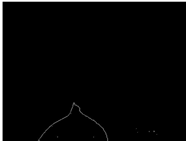
Fig. S5. Traced notch/crack profile by applying the Sobel method.
