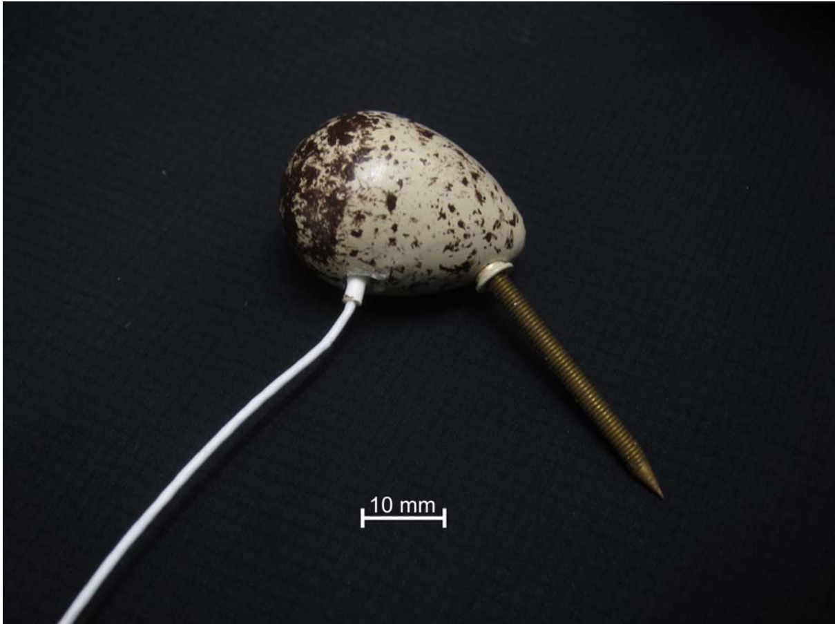
Picture S3. Fake-egg with inserted MSR temperature-probe and with attachment pin to secure it in the nest. For higher conductance the hole in the egg, which contains the probe, is filled with heat-sink grease. The probe is secured with silicon.
