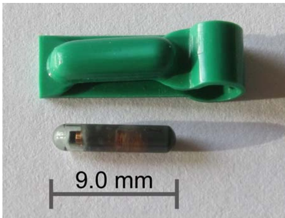
Picture S1. Glass passive-integrated RFID tag embedded in a flag. The flag was put on the tarsus and the part that sticks out was closed using an AA battery powered soldering device (Weller BP645).
