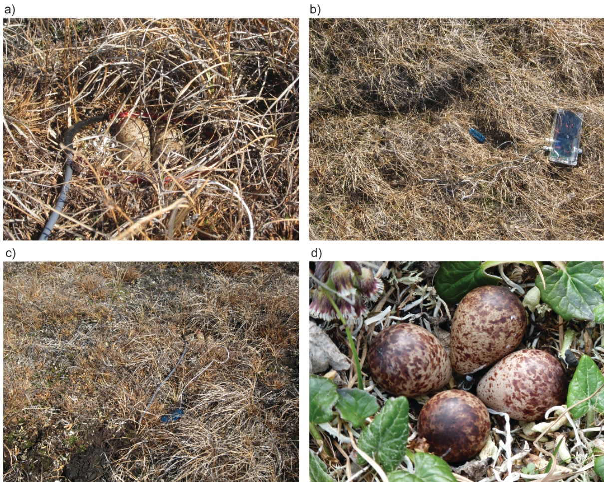
Picture S2. Incubation monitoring system. (a) The red RFID-coil detected the bird's identity. The coil was connected to the RFID reader (plastic box), placed either next to the nest in the open (b) or hidden in the vegetation (c). Data were processed by a custom board (Calima Engineering, http://www.calima.de ) equipped with an EFM32-Gecko microcontroller (Energy-Micro, http://www.energymicro.com/ ) and stored on a 2 GB SanDisk Standard SD card. Electricity to run the system came from 6 or 12 standard AA batteries. (d) Tiny-Tag temperature probe, positioned between the eggs. This probe registered temperature in the nest (in 2 min intervals), and therefore allowed to differentiate between incubation and non-incubation. Alternatively, we used an MSR fake-egg temperature probe, connected to a data-logger (blue device in b, c). This device registered both incubation temperature and tundra temperature (every 5 s).
