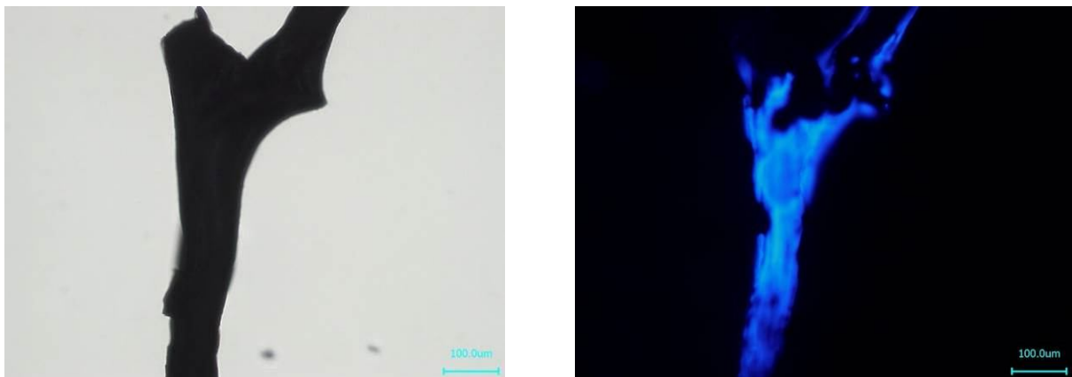
Figure S17. | Light (left) and fluorescence (right) microscopy images of the I. basta chitinous skeleton sample heated at 300°C, cleaned using 3M HCl and stained after that with CFW. Light exposure time: 1/10 s.
