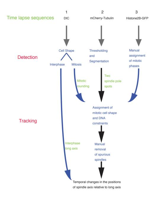
A Flow diagram of Spindle pole detection, tracking and spindle axis determination
