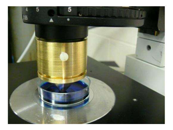
Figure S1. Condenser attachment for TTD imaging in cell culture dishes. See main text for details.
