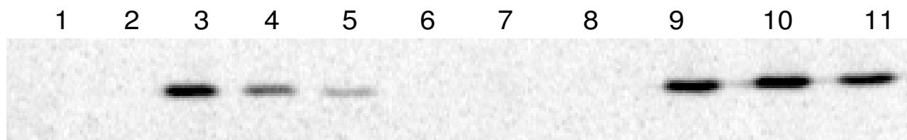
Figure S2. Purification of DHFR containing amino acid A at position 16 by successive chromatographies on Ni-NTA and DEAE-Sepharose CL-6B columns. Lane 1, flow through from Ni-NTA column; lane 2, elution with 10 mM imidazole; lane 3, first elution with 150 mM imidazole; lane 4, second elution with 150 mM imidazole; lane 5, third elution with 150 mM imidazole; lane 6, flow through from the DEAE-Sepharose CL-6B column; lane 7, elution with 100 mM NaCl; lane 8, elution with 200 mM NaCl; lane 9, first elution with 300 mM NaCl; lane 10, second elution with 300 mM NaCl; lane 11, third elution with 300 mM NaCl.
