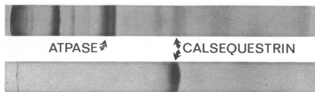
FIG. 1. Polyacrylamide gel electrophoresis in sodium dodecyl sulfate. The upper gel is sarcoplasmic reticulum, the lower gel is purified Calsequestrin.
