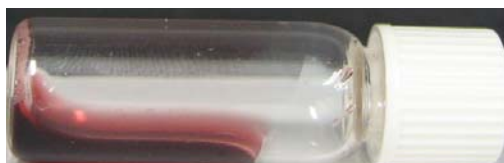
Figure S5. After the addition of 20 U/mL of ALP into the solution of 2d (0.6 wt%, pH 7.4), optical image shows that the resulting solution of 3d fails to form a hydrogel (or even a viscous solution).
