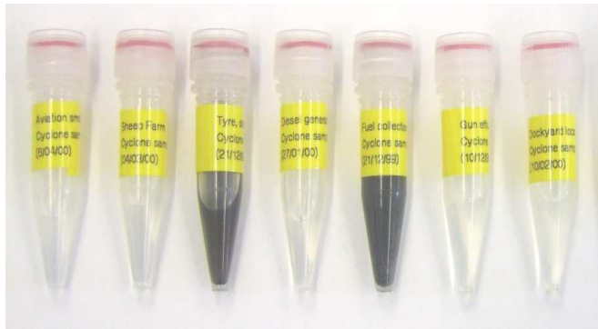
Figure S1. Buffer samples collected from a HWWC situated in seven different environmental scenarios. From left: Airfield; Sheep Farm; Burning Combustibles; Diesel Generator; Burning Fuel; Firing Range; Dockyard.
