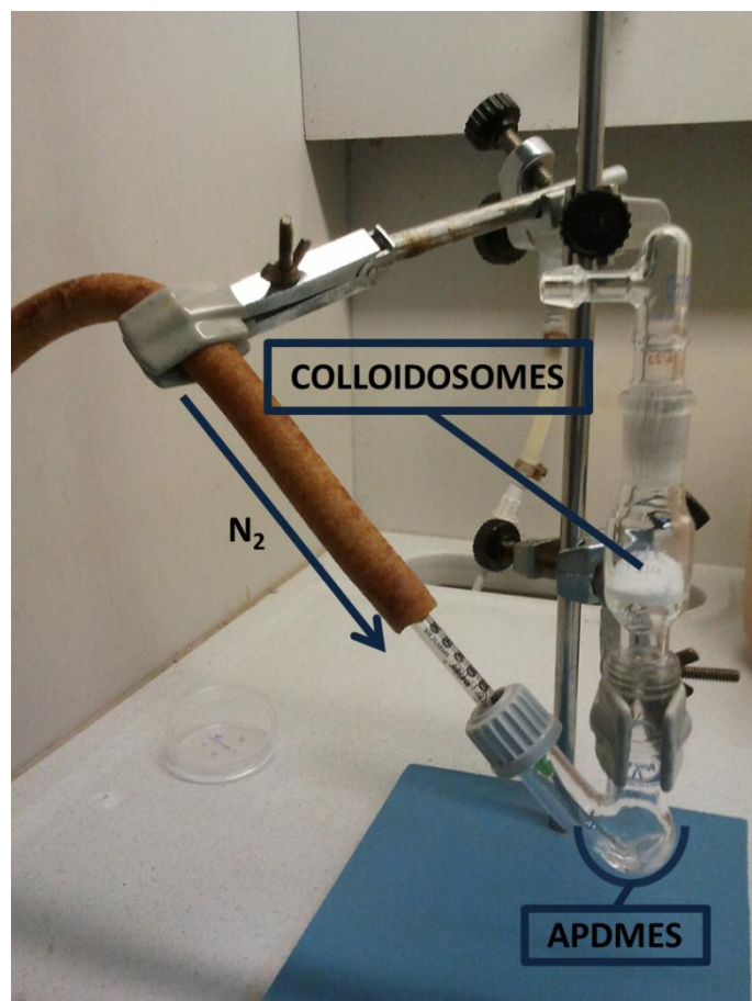
Figure S2. Experimental setup employed for the gas-phase silane deposition.
